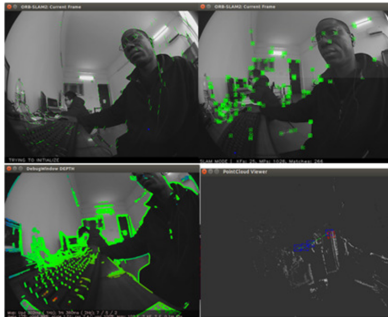
Figure 1. Combining Feature-based and Feature-less Method: Top left Trying to initialize on ORB-SLAM2. Top right Image initialized on ORB-SLAM2. Bottom left Keyframes with color-coded semi-dense depth map. Bottom right Pose-Graph with semi-dense depth maps.
