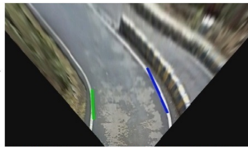
figure 8(b): Bird eye view showing only two Hough lines corresponding to each curve (lane). Problems due to noise and small curves were removed by using weighted centroid and slope filtering algorithms
