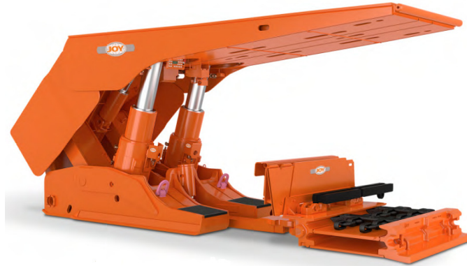
Fig. 1 Single unit of powered roof support ( www.joy.com ).
