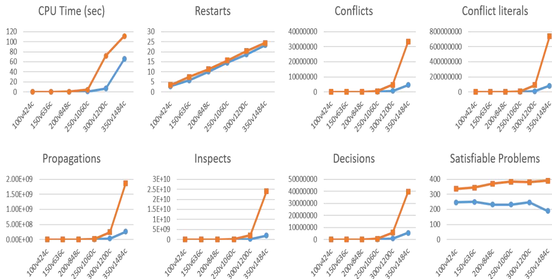
Figure 2: \alpha = 4.24 , 400 instances, Red: ETRSG, Blue: TSG. When more than 250 variables, ETRSG instances significantly outperform TSG instances in all aspects, except with slight outperformance in restart. ETRSG has a higher probability of generating solvable instances.
