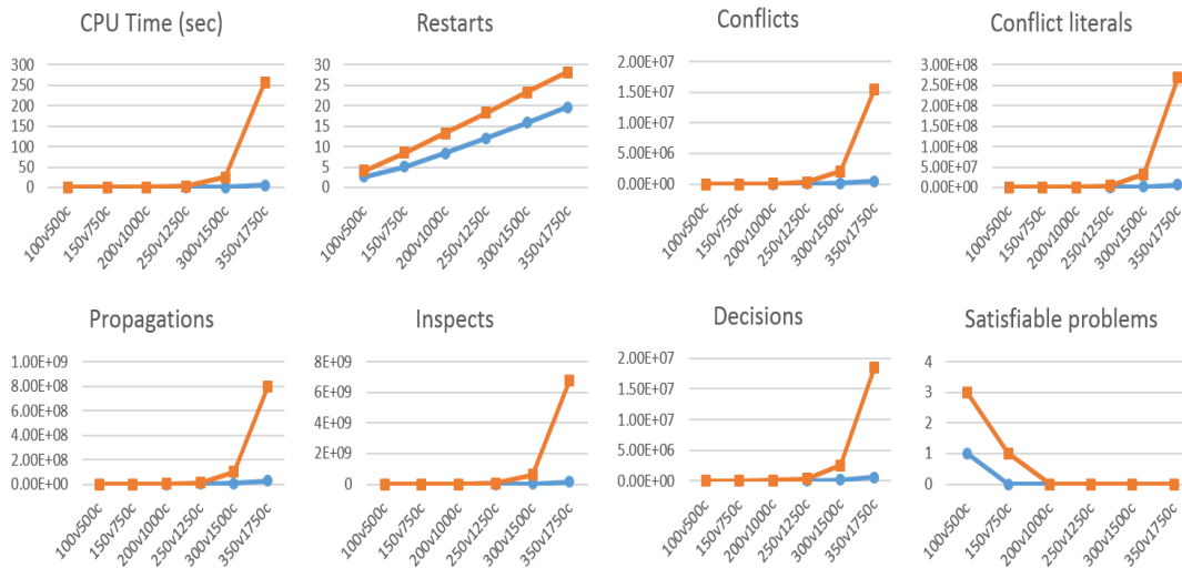
Figure 3: \alpha = 5 , 400 instances, Red: ETRSG, Blue: TSG. Similar to \alpha = 4.24 , but more significant in restart. The probability of generating solvable instances drops quickly to 0 for both since 5 is greater than the critical phase transition number.
