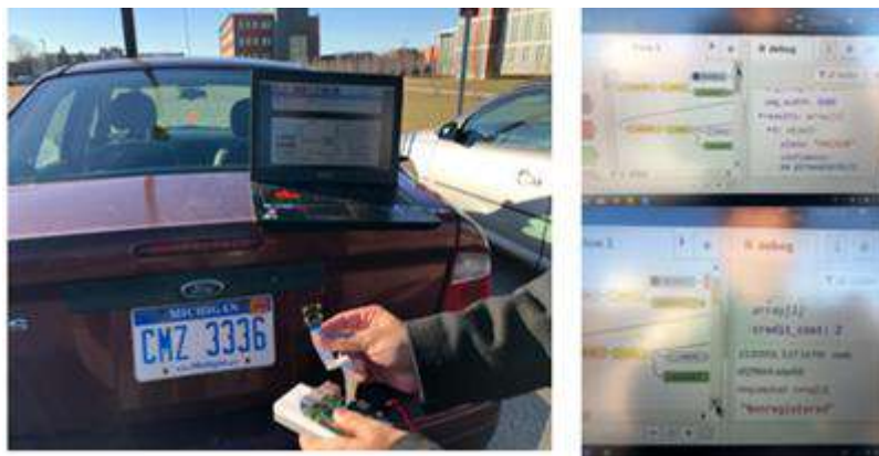
Fig 8: The picture shows the license of a different car and the license being recognized as unregistered.
