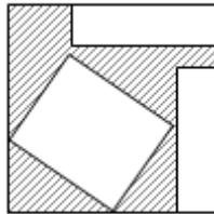
Figure 1. Non feasible shape by the shears
