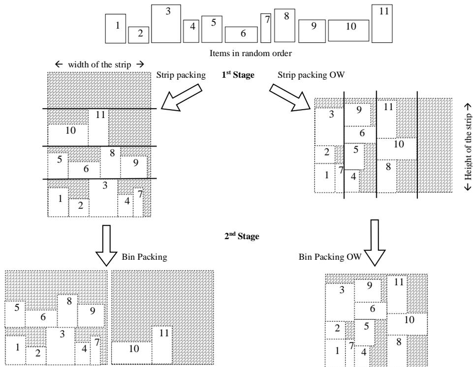
Figure 6. Our Approach 1<sup>st</sup> and 2<sup>nd</sup> stages: Classical Strip packing and Bin Packing vs. Optimization width Strip packing and Bin Packing
