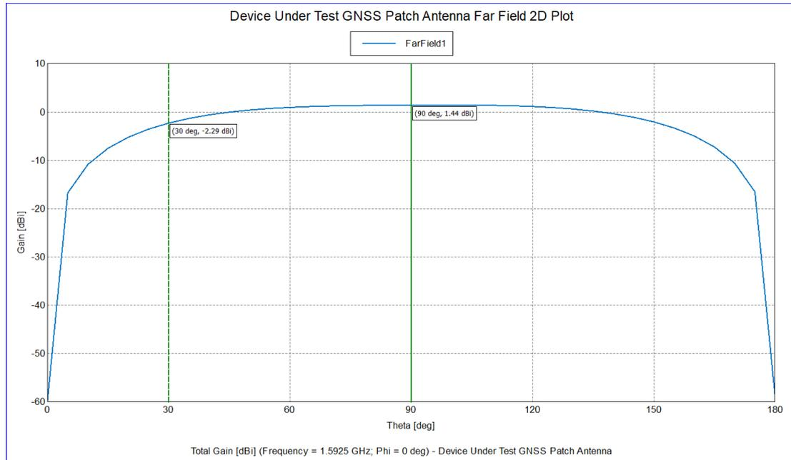
Figure 10. Patch antenna passive gain at 1.5925 GHz
