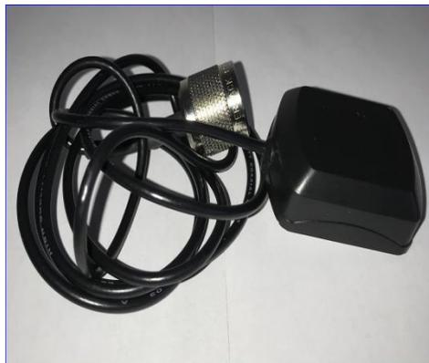
Figure 3. GPS Only Patch Antenna
