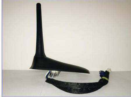
Figure 1. Dual Band Constellation GNSS Patch Antenna
