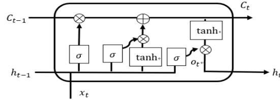
Figure 1. LSTM structure
