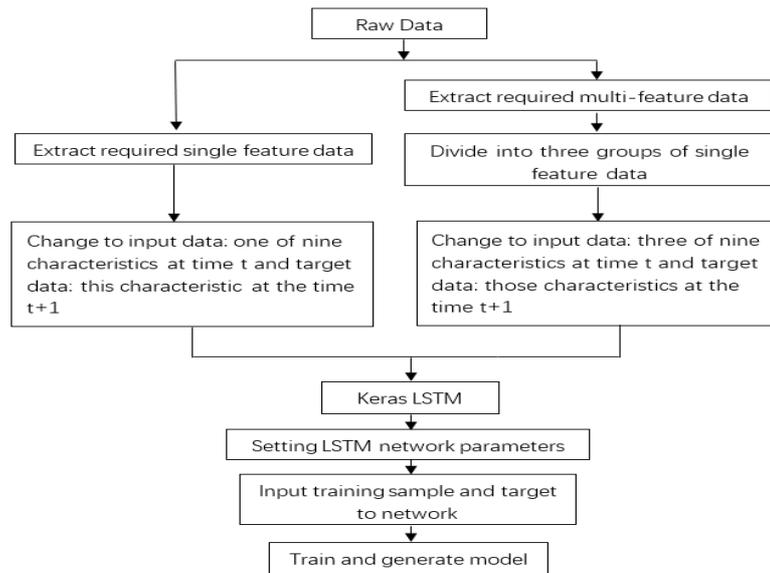
Figure 2. The flowchart of model establishment
