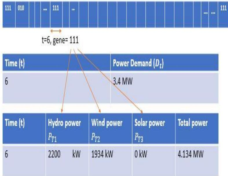
Fig. 3. Encoding scheme breakdown
