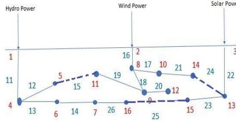
Fig. 5. Red numbers are nodes, Blue solid/dashed lines are line section active/opened, Blue numbers are line section number
