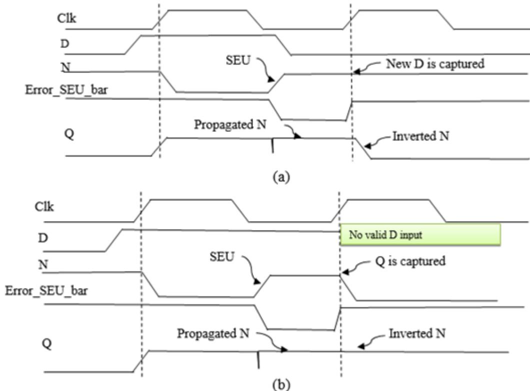
Figure 5. SETTOFF Operating principle [13]
