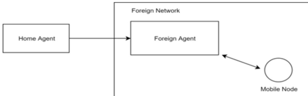
Figure 2. An Overhead View of IP Mobility Support for IPv4.
