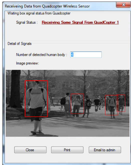
Figure 9. Application form of receiver on server when get some signal from quadcopter
