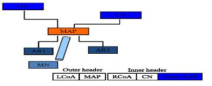
Fig.2 How MAP create tunnel for MN
