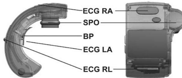
Fig. 2. Photograph of AMON Sensors: ECG, SPO<sub>2</sub>, and Blood Pressure (Courtesy of Anliker *et. al* [7])
