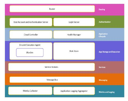
Figure 3. Cloud foundry components
