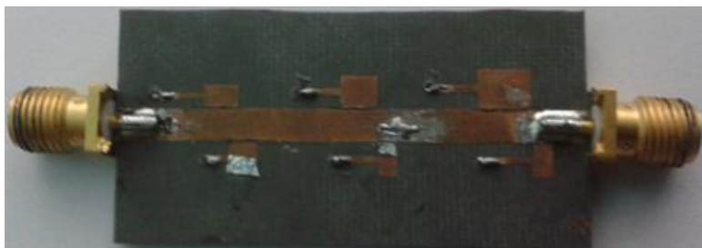
Fig 8: Fabricated Multiresonator circuit with all the resonators shorted
