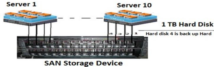
Figure 5. Servers and SAN storage device architecture
