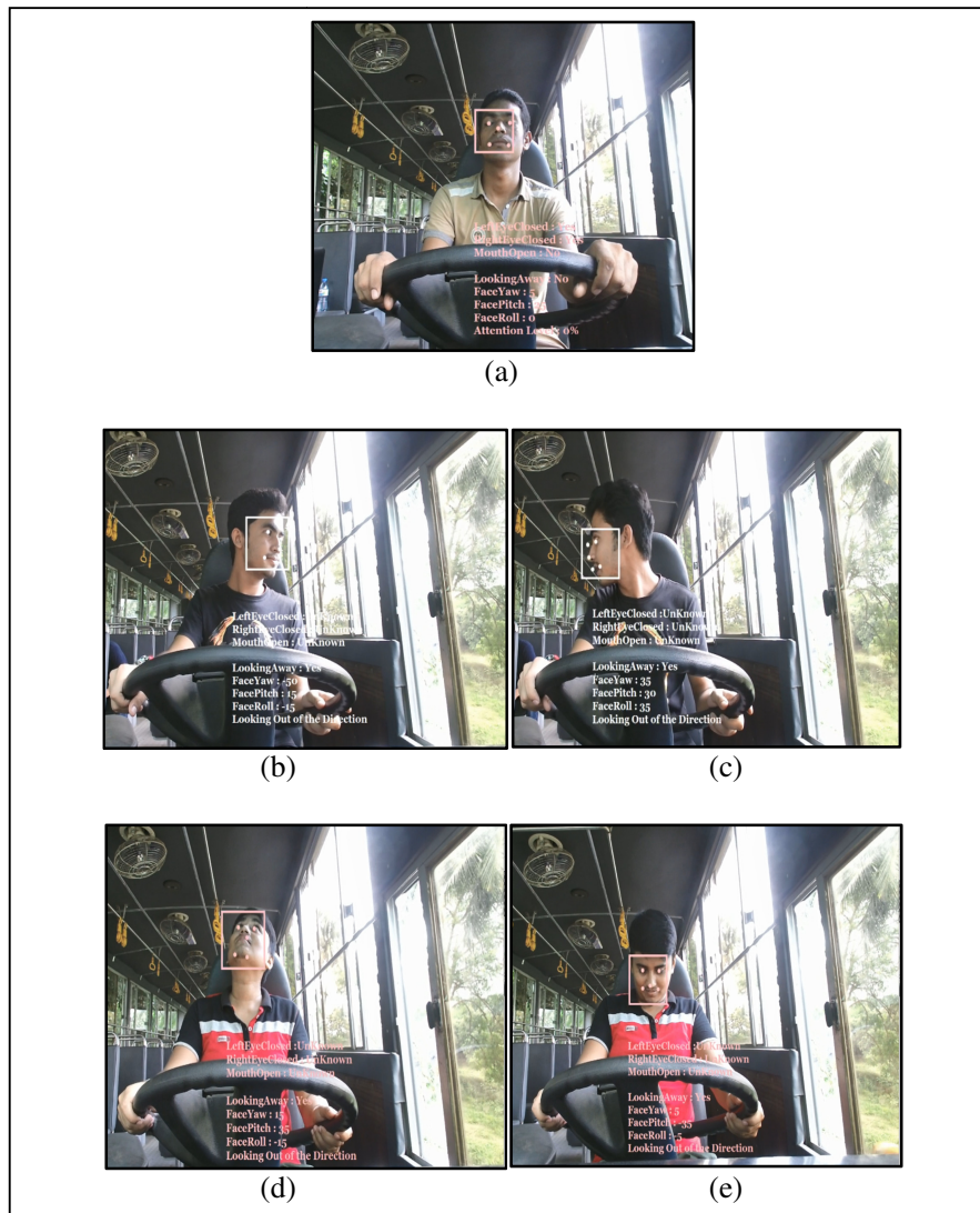
Figure. 5. Examples of alarm generating cases:(a) when both eyes are closed for 2 seconds or more than 2 seconds,(b) looking out of the direction (left side),(c) looking out of the direction (right side),(d) looking out of the direction (up) and(e) looking out of the direction (down)
