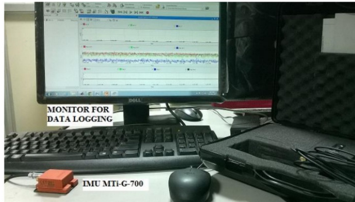
Figure 4: Experimental arrangement of Xsens MTi-G-700
