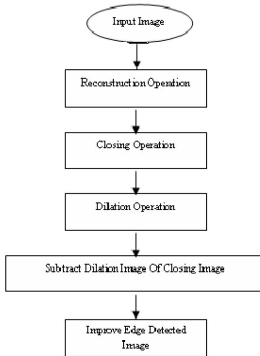
Fig.4.Flow chart of purposed algorithm
