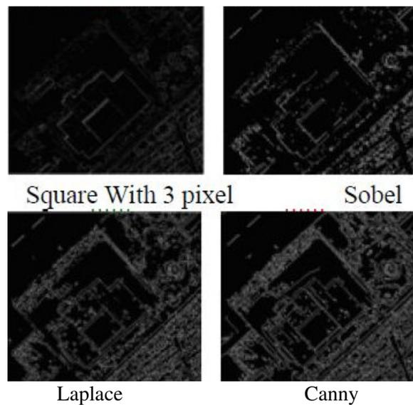
Fig5.Purpose Algorithm Result and Comparison Various Structure Elements with Various Pixel Number And Sobel, Laplace, Canny Operators
