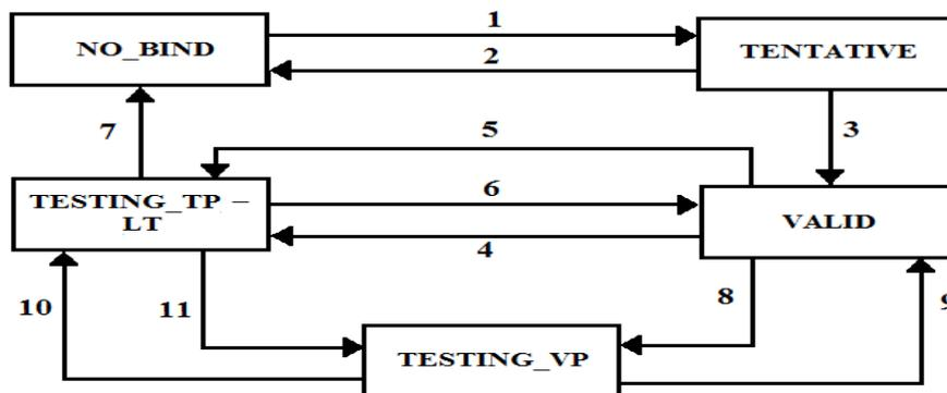
Figure 8: The finite state machine of the FCFS SAVI method.
