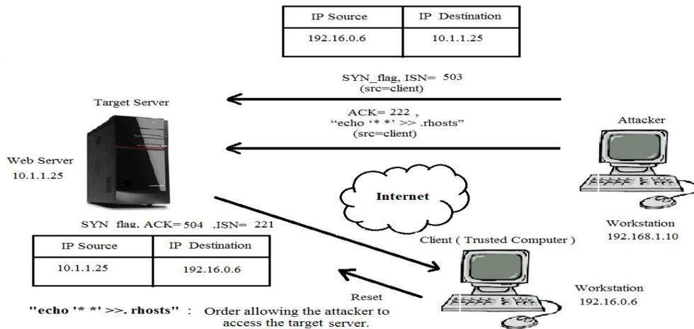
Figure 2 : Stages of the IP Spoofing attack.
