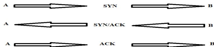
Figure 1: The phases of the establishment of a TCP connection.
