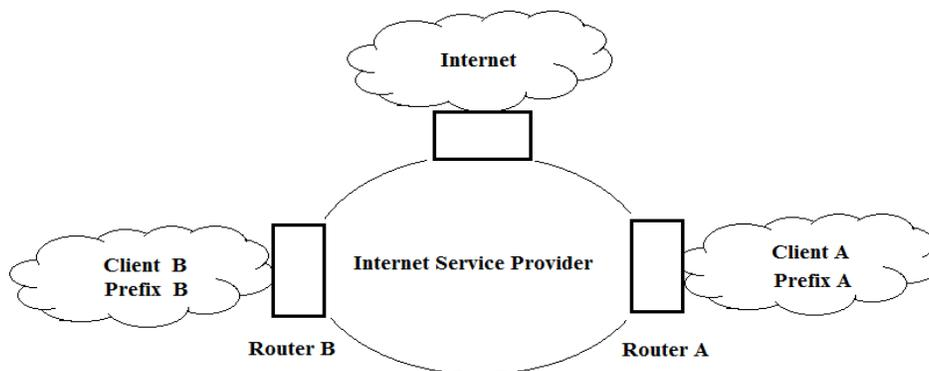
Figure 3 : Architecture using the technique "Network Ingress Filtering".
