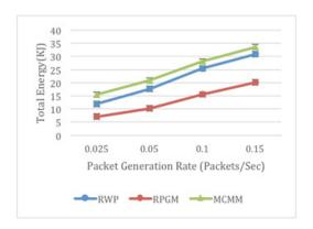
Figure 10: Effect of Traffic Load on Total Energy Consumption When using RWP, RPGM & MCMM.
