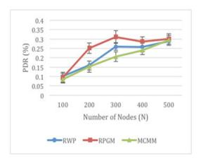
Figure 2: Effect of network density on PDR when using RWP, RPGM & MCMM.
