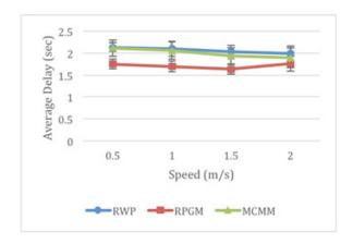
Figure 6: Average end-to-end delay vs Speed when using RWP, RPGM & MCMM.
