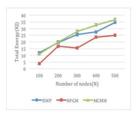
Figure 4: Effect of Network Density on Total Energy Consumption When using RWP, RPGM & MCMM.
