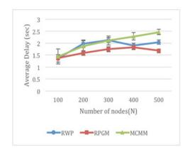
Figure 3: Effect of network density on the average end-to-end delay When using RWP, RPGM & MCMM.
