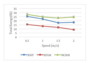
Figure 7: Total Energy Consumption Vs Speed when using RWP, RPGM & MCMM.
