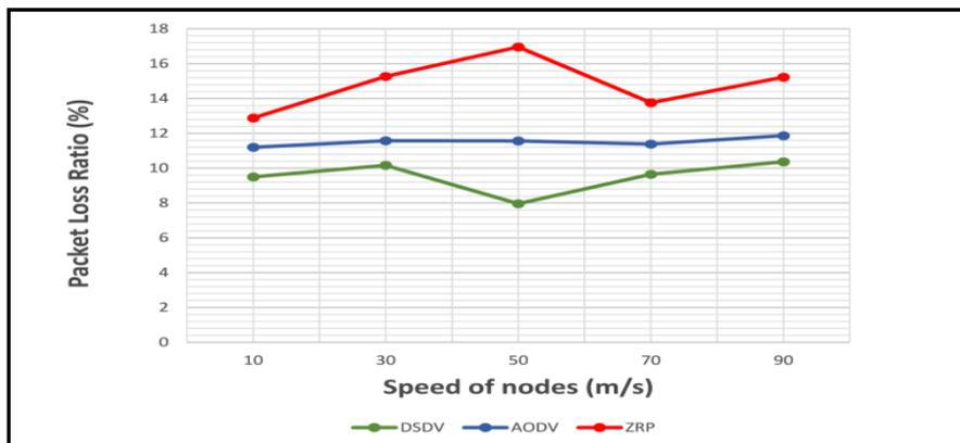
Figure 10. Packet Loss Ratio vs speed of nodes for 100 nodes model
