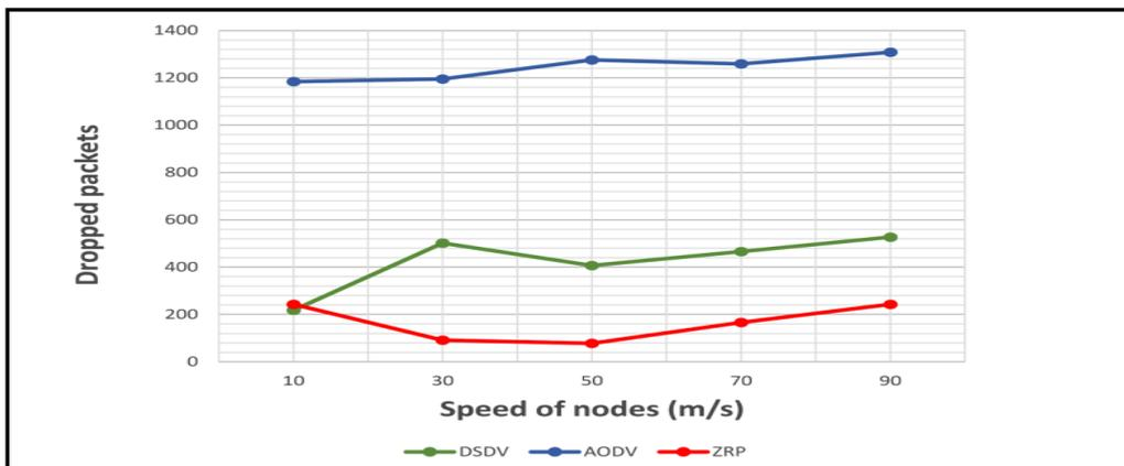
Figure 12. Dropped Packets vs Speed of nodes for 100 nodes model
