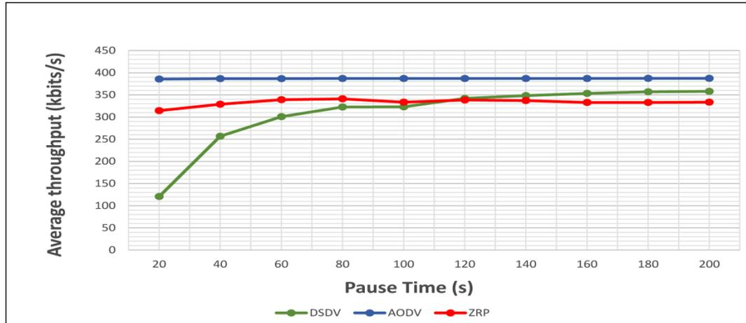
Figure 13. Average Throughput vs Pause Time for the 10 nodes model
