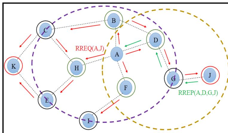
Figure 6. ZRP Routing Protocol Transmission
