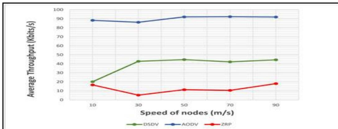
Figure 8. Average Throughput vs Speed of nodes for 100 nodes model
