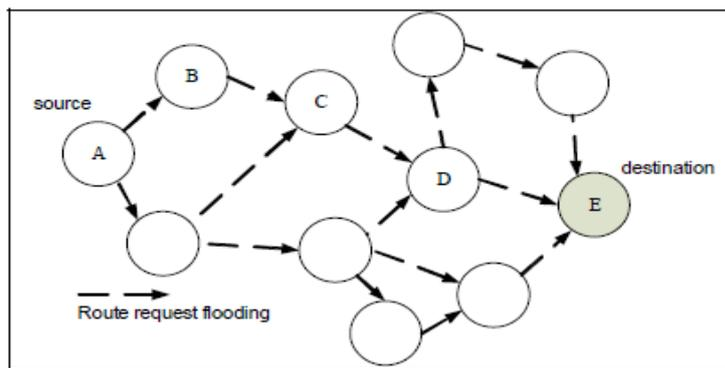
Figure 4. Route Request flooding
