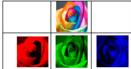
Figure 2. Separation of Image into R, G and B plane
