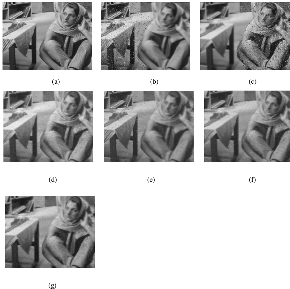
Figure 7. (a) Reference image. (b) Source image1: Right part of image has salt and pepper noise and the left part of it is blurred. (c) Source image 2: Left part of image has salt and pepper noise and the right part of it is blurred. (d) Result image with FAR method. (e) Result image with DS_MS method [2]. (f) Result image with Han's method [6].(g) Result image with our method.
