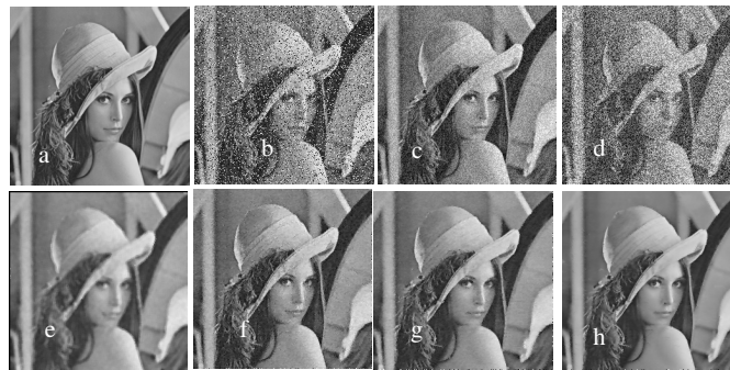
Fig.5 Subjective performance illustration of the proposed filtering technique compared with existing technique: (a) Original Lena image, (b) Lena image Corrupted by 10% impulse noise and uniform noise with zero mean and \sigma=200 , (c) Restored by median filter, (d) Restored by midpoint filter, (e) Restored by ATMPF (f) Restored by MAATMPF, (g) Restored by NDBN filter and (h) Restored by proposed algorithm.
