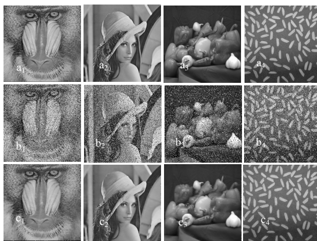
Fig. 8 Performance of test images: (a 1,2 and 4) original images,(b 1,2 and 4) images corrupted with 10% of impulse noise and uniform noise with \sigma=200 and (d 1, 2 and 4) images enhanced by proposed filter
