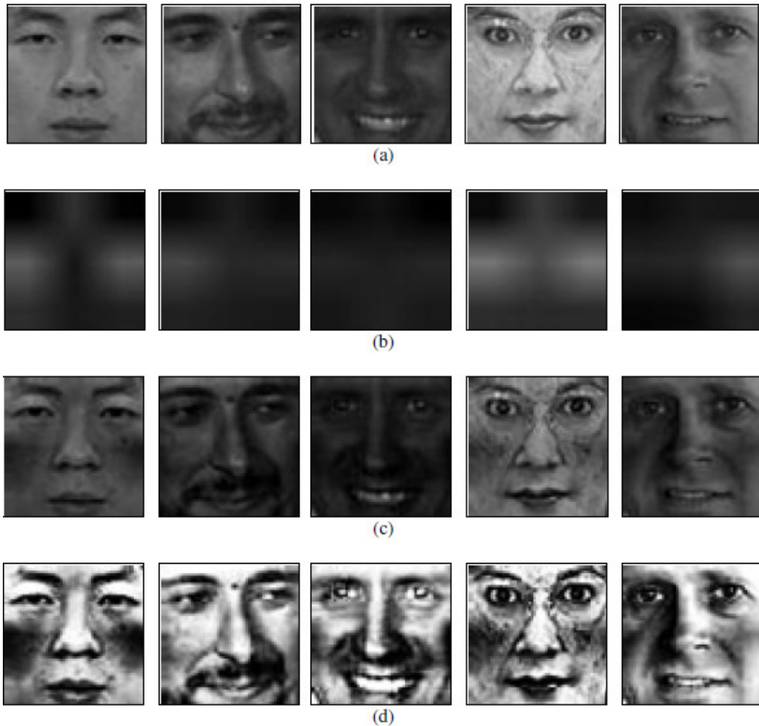
Figure 2. Five examples of illumination correction. (a) original face images (60x60), (b) minimal brightness planes, (c) illumination-corrected images by subtracting (b) from (a), (d) images enhanced by histogram equalization.
