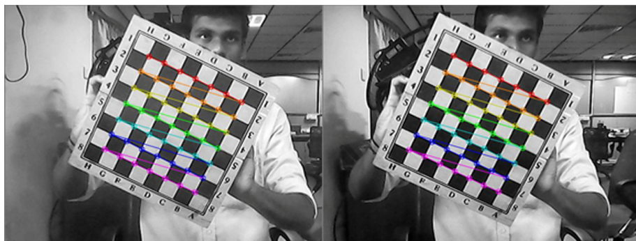
Figure 3. Stereo camera and rig calibration using chessboard as a calibrating object. Detected chessboard corners are marked in simultaneously taken left and right images.
