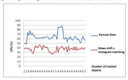
(b) Graph of CPU resources used when tracking multiple-targets using the particle filter and our proposed method.
