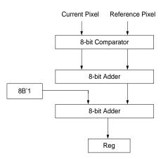
Figure 1: AD circuit block diagram
