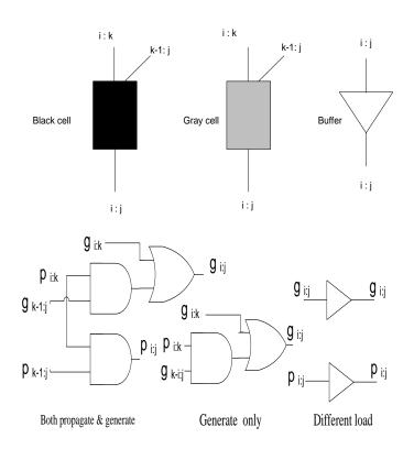
Figure 3 Cell definitions for parallel-prefix scheme [10]
