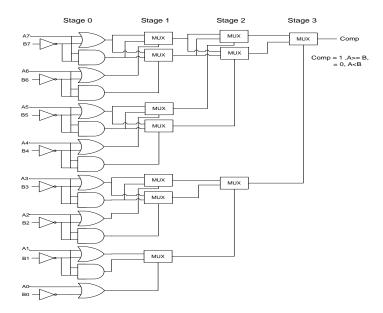
Figure 7 Modified comparator architecture
