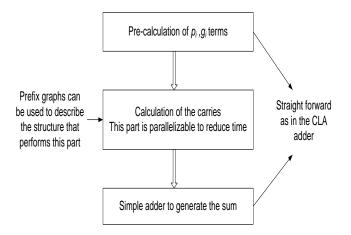
Figure 2: Parallel Prefix Adder stages
