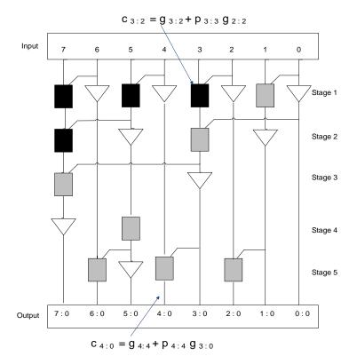
Figure 4 : 8-bit Brent-Kung adder(BKA) tree [13]
