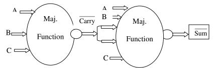
Figure 10 Basic design approach for Majority Not function based full adder cell
