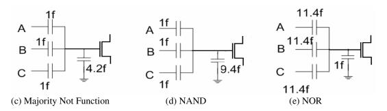
Figure 6. Dynamic CMOS MOSCAP (NAND, NOR and Majority-NOT) logic gate
