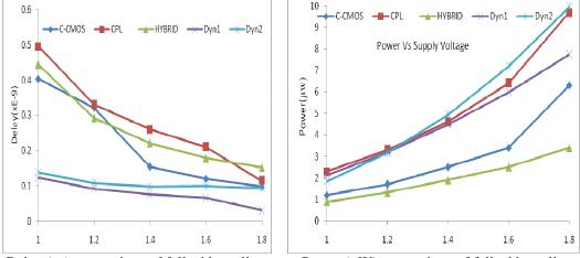
Delay (ns) comparison of full adder cells Figure 15 Delay & Power comparison of conventional full adder cells
