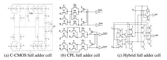
Figure1. Conventional Static full adders
