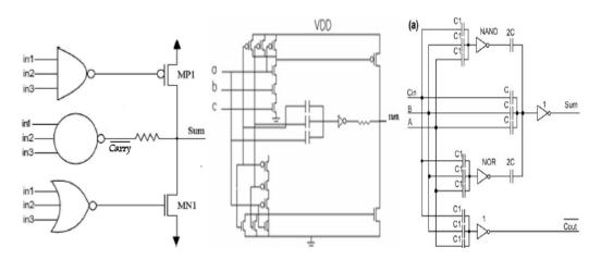
Figure 8 Basic design methodologies for Majority function based full adder circuit
