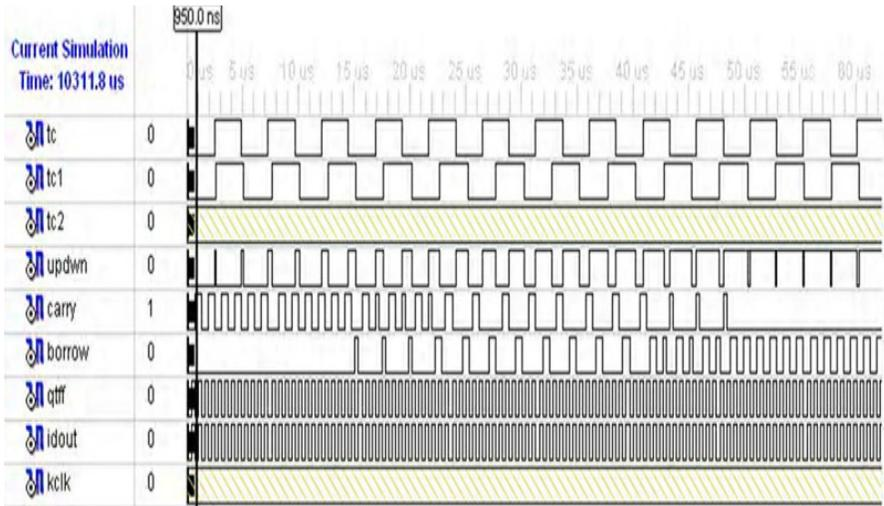
Figure 3. Simulation output of the ADPLL in locked condition at  $f = 199 \text{ kHz}$
