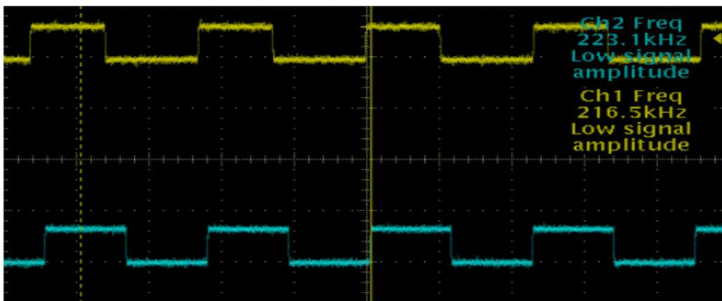
Figure 11. FPGA output of the ADPLL (ripple reduction technique) in unlocked condition at  $f = 216$  kHz
