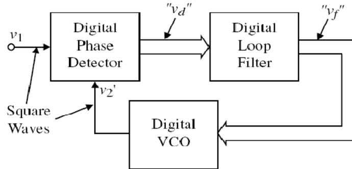
Figure 1. The basic block diagram of ADPLL
