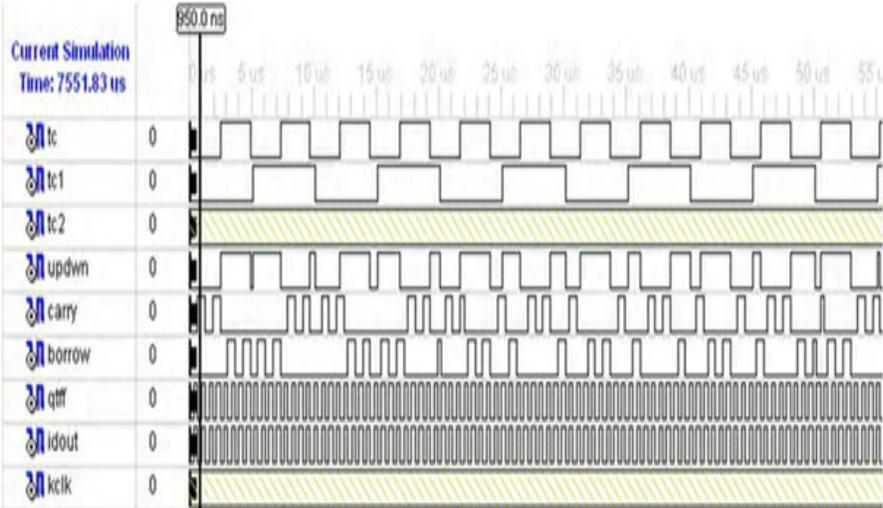
Figure 4. Simulation output of the ADPLL in unlocked condition at  $f = 200 \text{ kHz}$
