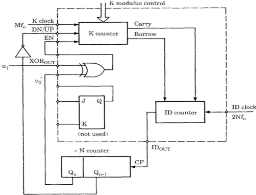
Figure 5. ADPLL design with ripple reduction technique.
