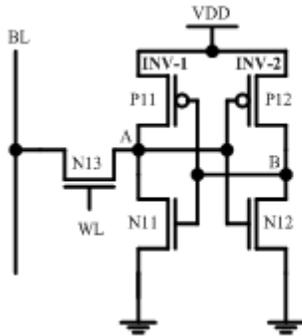
Figure 4. Simplified circuit diagram during the write operation.
