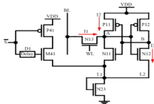
Figure 7. Simplified circuit diagram during the standby operation.
