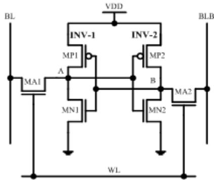
Figure 1. Circuit diagram of standard 6T SRAM cell
