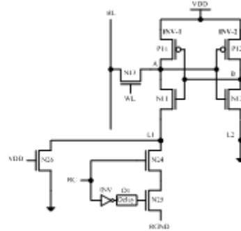
Figure 5. Simplified circuit diagram during the read operation.
