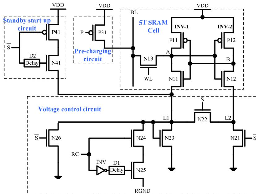
Figure 3. Circuit diagram of the proposed 5T SRAM cell
