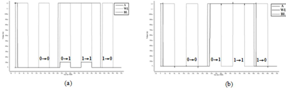
Figure 8. (a) Transient waveforms of a write failure in the traditional 5T SRAM cell, (b) Transient waveforms of a successful writing in the proposed 5T SRAM cell.
