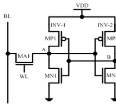
Figure 2. Circuit diagram of traditional 5T SRAM cell
