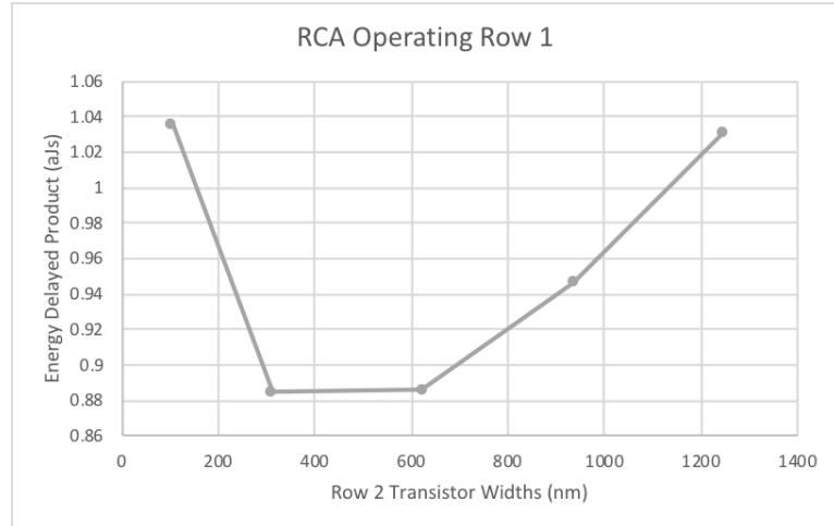
Figure 5. EDP Curve for the RCA Operating on Row 1 while the Multiplier is Sleeping on Row 2.
