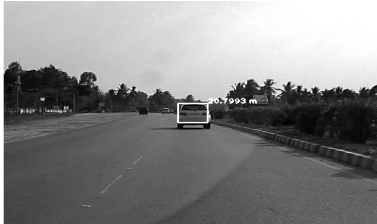
Figure 4. Distance computed using SFM
