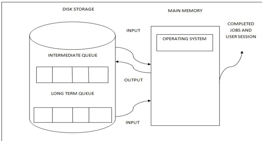
Figure 6. Swapping with Input and Output Operations
