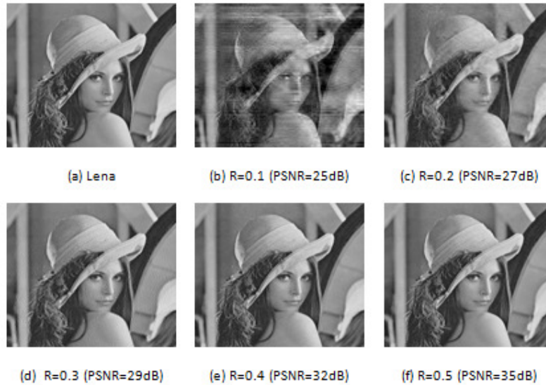
Figure 6. Demonstration of BStROMP with the same block size(32×32) but different sampling rate
