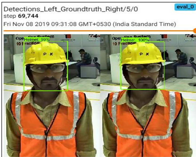
Figure 9. Bounding box detections in left and ground truth in right for images in validation set
