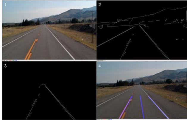
Figure 2: Lane Keep Assist Detections
