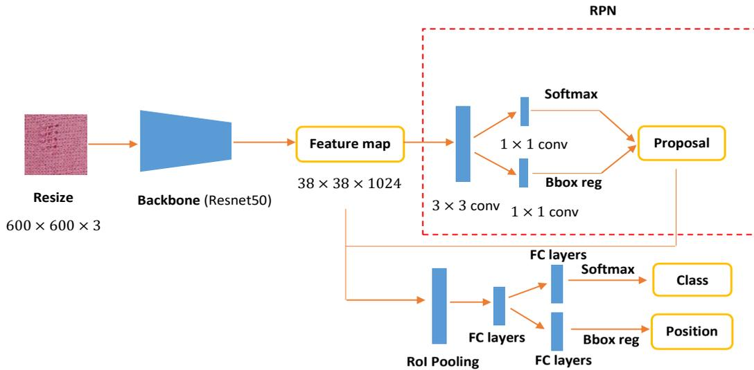
Fig 2. An illustration of Faster R-CNN model
