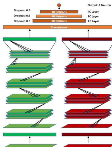
Figure 8. Model Architecture for Seg + Depth Multi-Channel CNN
