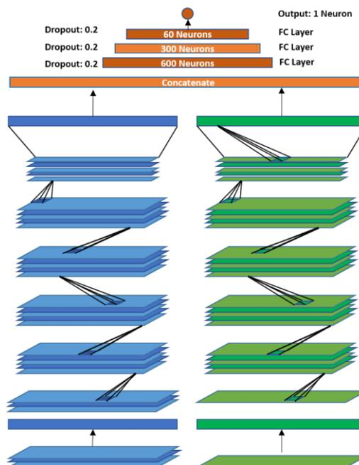
Figure 6. Model Architecture for RGB + Seg Multi-Channel CNN
