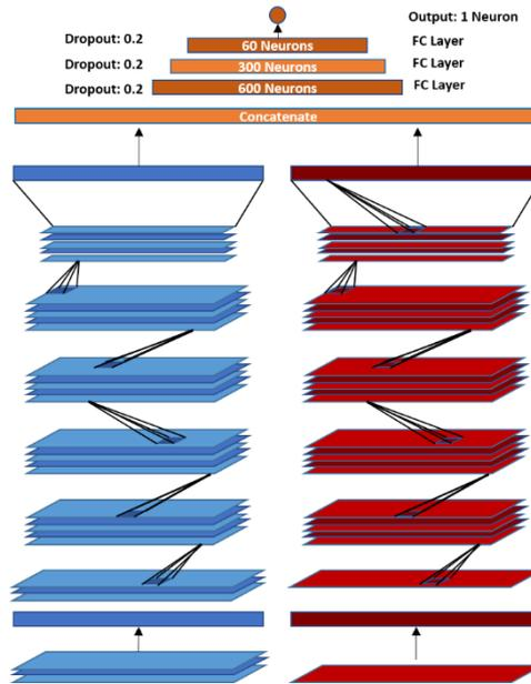
Figure 7. Model Architecture for RGB + Depth Multi-Channel CNN
