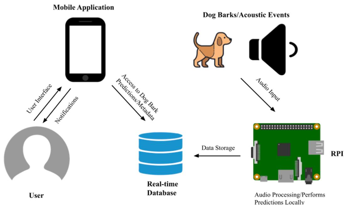
Figure 1. Graphic Representation of the solution
