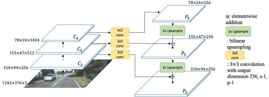
Figure 3. The RGB stream backbone ResNet-50-FPN
