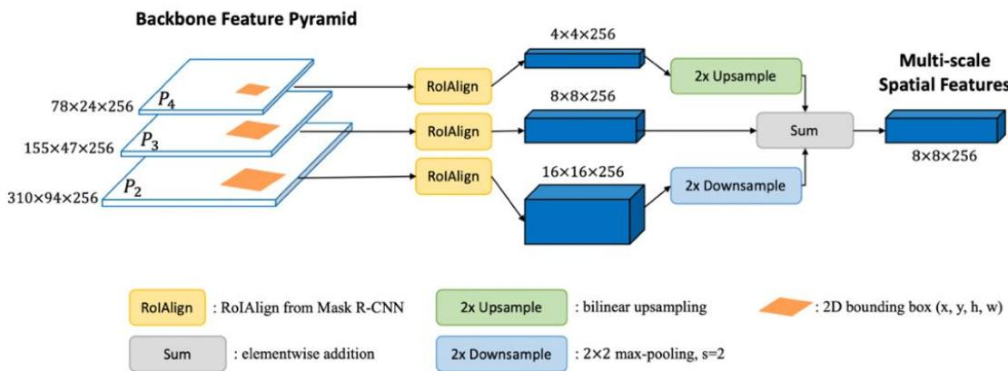
Figure 6. Architecture of multi-scale feature aggregation module
