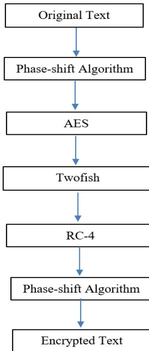
Figure 1. Encryption Process
