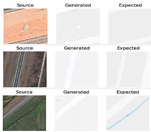
Figure 3. Pix2Pix model output of plausible maps from satellite images. Generated maps are shown compared to ground truth or expected output from Google Maps API.
