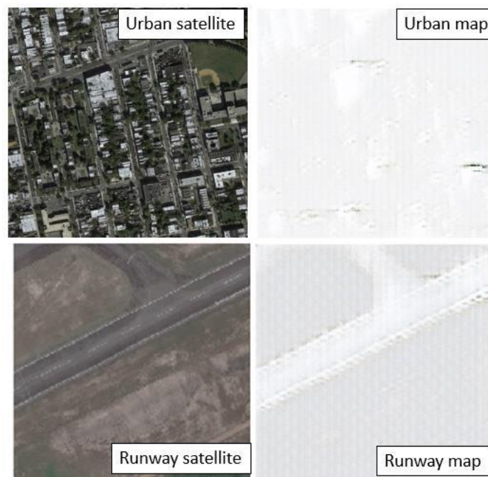
Figure 5. Comparison of multi- and single-class Pix2Pix generated maps. The urban satellite image generates a lower resolution map lacking the features expected and the single-class map shows the simple runway outline as expected.
