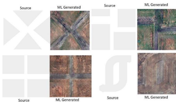
Figure 9. Example sketched maps and the corresponding generated satellite images. The Pix2Pix model renders plausible synthetic satellite data from hand sketches for runways.
