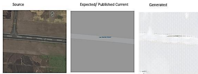
Figure 10. Faulty Google Map API runway map for Lae Nadzab Airport, Papua New Guinea (AYNZ). The satellite image shows a three-way intersection, which is correctly captured by the Pix2Pix model but incorrectly shown in the published map.
