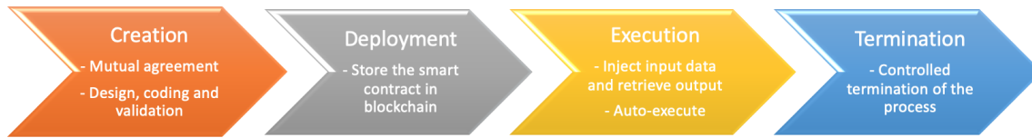
Figure 4. The life cycle of a smart contract, the creation-deployment-execution-termination.
