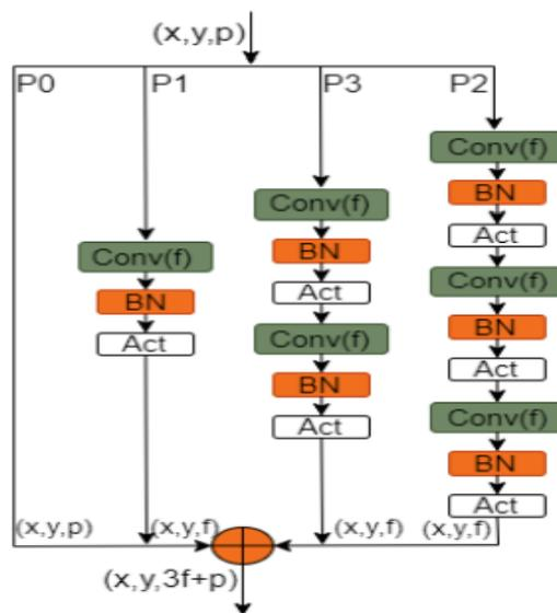
Figure 2. Schematic diagram of the M-Block
