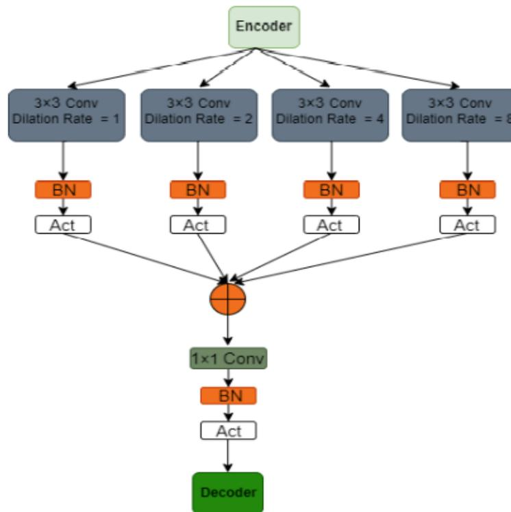
Figure 3. Schematic diagram of the dilated Block
