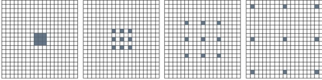
Figure 4. Dilated convolution with 3x3 Kernel with a dilation rate of 1, 2, 4 and 8
