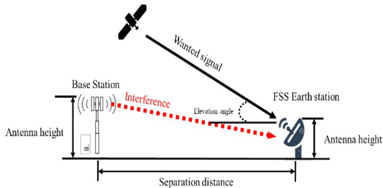
Figure 2. interference from adjacent band 5G emission
