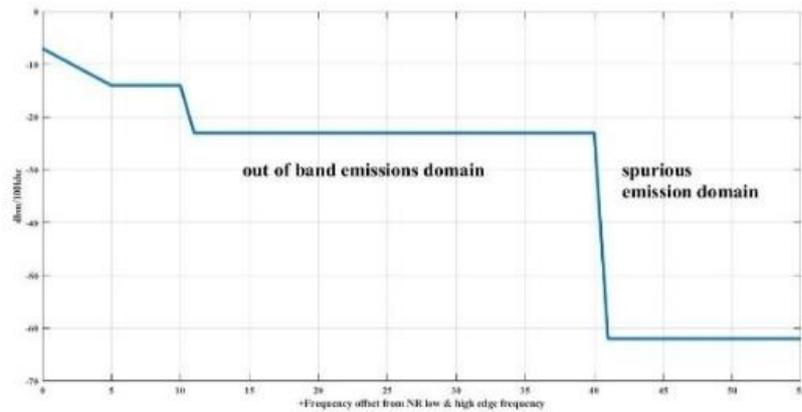
Figure 3. Unwanted emissions limits [7] (dBm/100 kHz)
