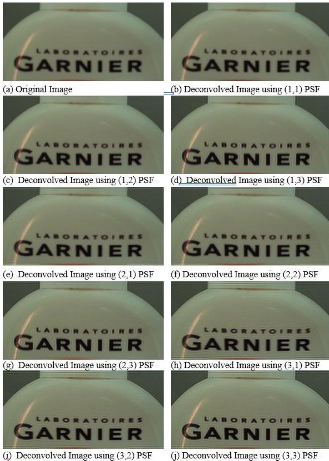
Figure 3. Sample image which underwent blind deconvolution using different PSFs as indicated
