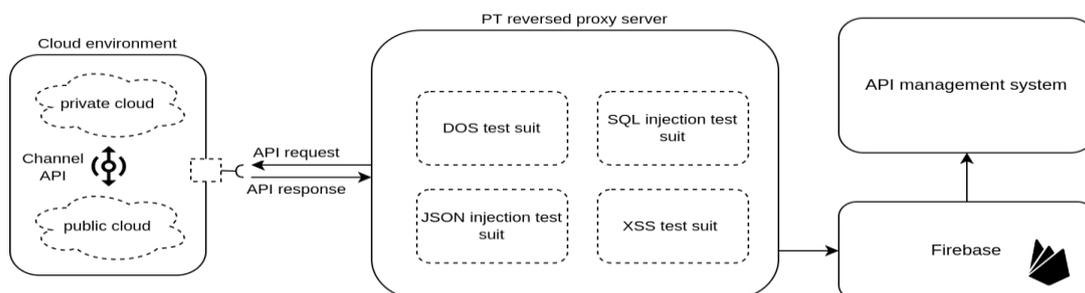
Figure 1. High-level architecture
