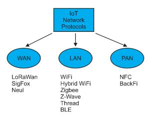
Figure 1. Common IoT network protocols [2]
