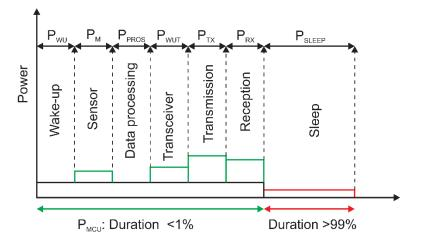
Figure 5. Power consumption model of sensor node
