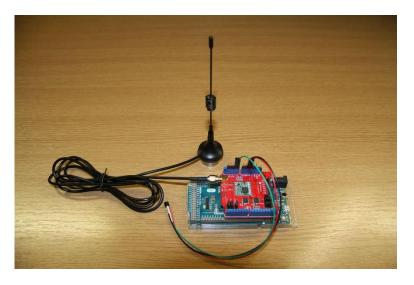
Figure 8. Arduino Due with Dragino LoRa shield and antenna
