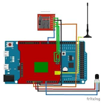
Figure 9. The schematic representation of the slave
