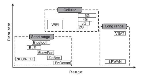
Figure 2. Comparison between various communication protocols in IoT [3]
