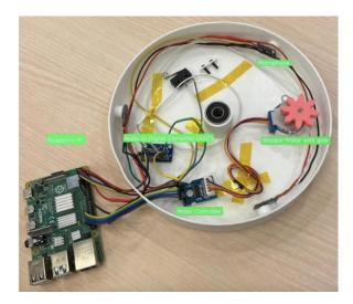
Figure 2. Overview of the components of the Circle of Command
